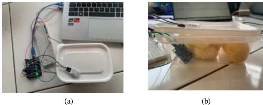
Figure 4. Prototype of Arduino Uno-Based Tape Fermentation Tool (a) Top view (b) Side view
